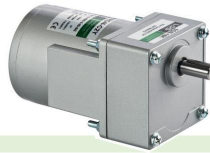
The Reversible Motor is designed for start/stop operations with changes of direction frequently. It is rated at 30 minutes while used in this fashion. It uses a simple damping brake to slow the motor quickly to be able to change direction efficiently. This generates heat when the motor is frequently changing direction which is why all reversible motors are rated for 30 minutes only. (But when large stored torque is required, model with electromagnetic brake should be used).
