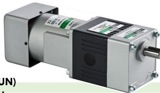
The DC 24V Clutch and Brake motor use a high precision, highly responsive clutch & brake for frequent start/stop operation. When the brake is in use, the clutch will separate the link from the brake, so there are no overruns, making positioning precise and accurate.
