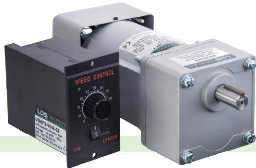
Variable Speed Motor uses an Induction Motor with a modular tacho-generator fitted to the rear of the motor. The tacho-generator is made of a magnet connected directly to the motor shaft and a stator coil that detects the magnetic poles, and generates an AC voltage at 12 cycles per revolution. The motor can run in either forward or reverse directions. It has independent powerful cooling fan to cool down motor in order to achieve longer lifespan.
