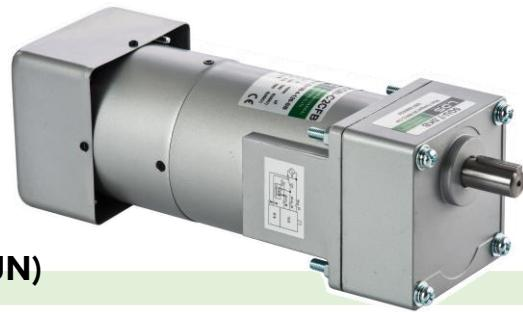
Electromagnetic Brake motor is ideal for vertical application in which the load must be held. It's a load-holding brake motor with a power off activated type electromagnetic brake, where the motor stops instantaneously when the power is cut off, while still holding the load in position (optimal solution for emergency brakes and vertical load applications).
