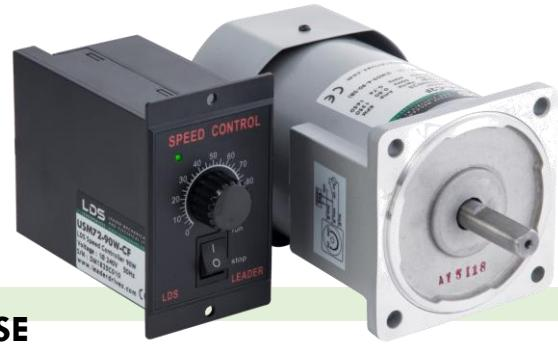
Variable Speed Motor uses an Induction Motor with a modular tacho-generator fitted to the rear of the motor. The tacho-generator is made of a magnet connected directly to the motor shaft and a stator coil that detects the magnetic poles, and generates an AC voltage at 12 cycles per revolution. The motor can run in either forward or reverse directions. It has independent powerful cooling fan to cool down motor in order to achieve longer lifespan.
