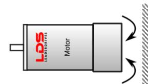
On installation, the mounting of the motor must allow a free-flow of cooling air over the surface of the motor (leave a minimum 20~30mm space from the rear cover of the motor).
