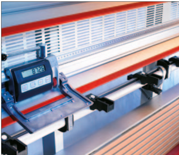
Direct display of measured values with a vertical panel saw ...
